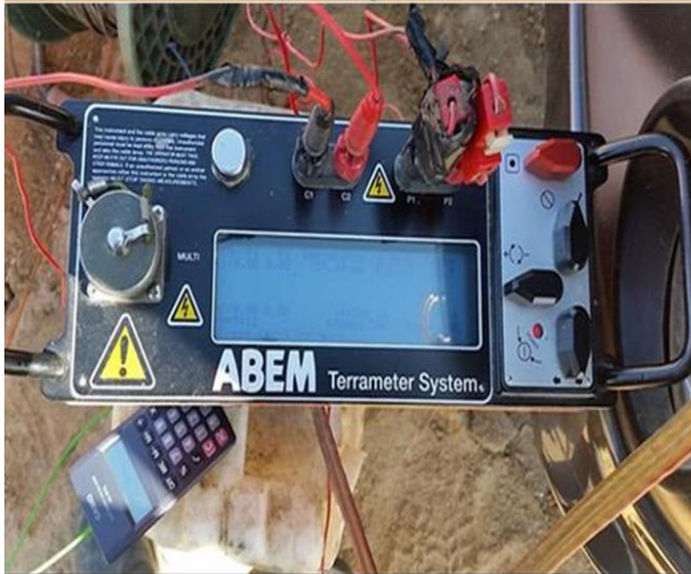
Figure 4. A conventional set-up of the earth resistivity meter geoelectrical resistivity field observations (after Robinson and Coruh, 1988).
